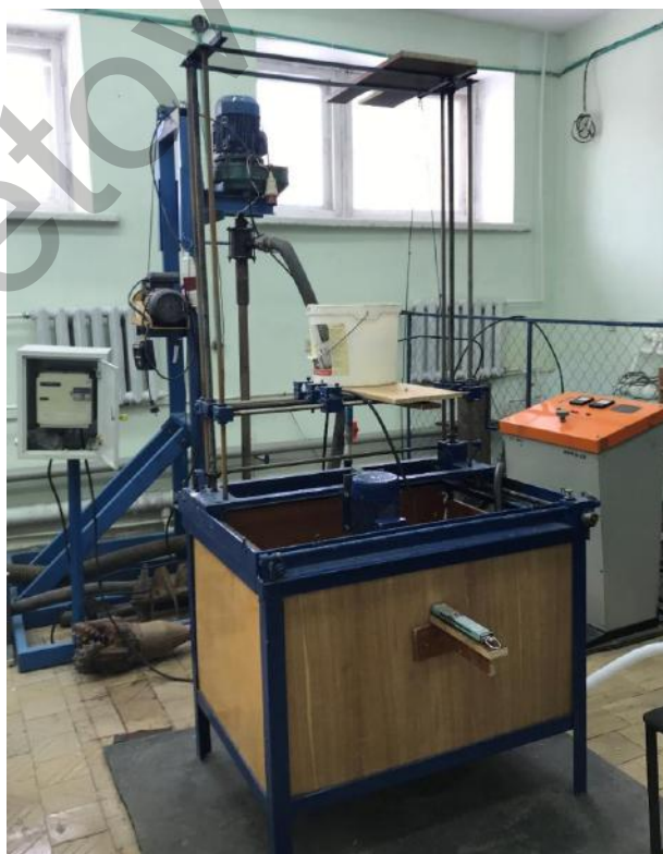
Fig.1. General view of the experimental setup for determining the flow rate through throttle holes.
