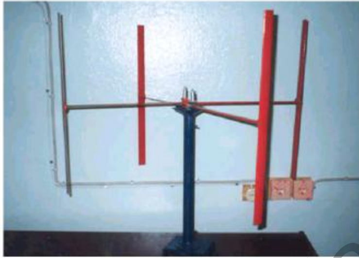
Fig. 7. An acting laboratory model of a Bi-Darrie turbine.
